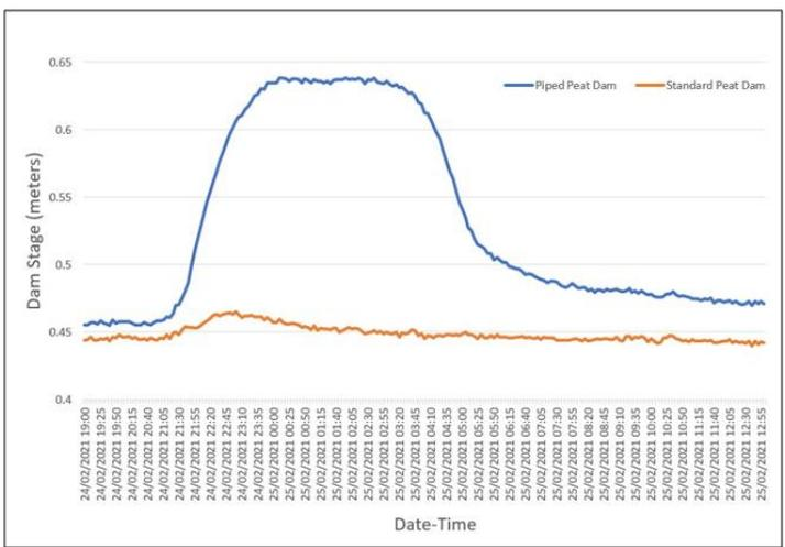
Piped peat dam (blue) and standard peat dam (orange) stage change during a storm
